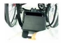
Place the battery pack in to the battery tray as shown in the photograph. Secure the battery pack on its tray.
