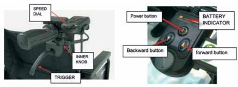
Please note there is a 2-second delay when starting up the PS-HA HD before the wheel will move. Wait 2 seconds before squeezing the trigger.
