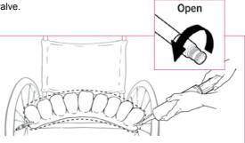
5. Pinch the rubber nozzle of the hand pump and close the inflation valve completely. Remove the hand pump.
